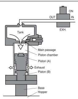
A large quantity of air accumulated in the tank flows through the main passage into the piston chamber. Then piston (A) moves at high speed to strike against piston (B), and thus vibration is transmitted through the base to the hopper.
