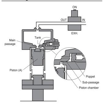
When the 3-port solenoid valve remains ON, air flows into the tank. When the pressure reaches the specified value, the poppet opens, the air passes through the sub-passage and flows into the piston chamber to move piston (A), and thus the main passage opens.
