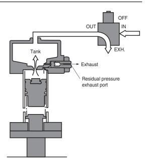
When the 3-port solenoid valve is turned OFF, the air inside the tank and cylinder is exhausted through the exhaust port of the solenoid valve and residual pressure exhaust port. Then piston (A) and poppet return to their initial condition.
