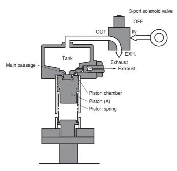
When the 3-port solenoid valve remains OFF, the tank and piston chamber are under atmospheric pressure, piston (A) is locked by a spring, and thus the main passage is closed.
